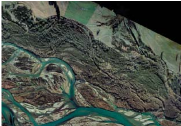
Fig 7: This image shows the same river reach in 2001. The braiding of the river has reduced as a result of upstream hydro development and subsequent flood reduction, river engineering works, in particular willow planting, and farming activities encroaching onto the fairway.
